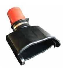
Oval rubber nozzle with 4.13" x 8.26" suction opening and 30° hose coupling with fully tight manual closing valve, probe for C.O. test and fixing clip with vulcanized rubber end.
