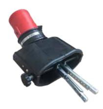
Oval rubber nozzle with 4.13" x 8.26" suction opening and 30° hose coupling with fully tight manual closing valve, probe for C.O. test and internal expanding grip with adjustable beaks.
