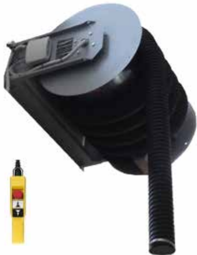
Electric recoil hose reel with wired buttons for exhaust extraction complete with crushproof flexible hose resistant up to 400°F and automatic electric stopper. Internal winding motor single phase 110V.
