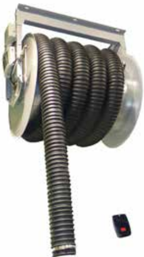
Electric recoil hose reel with remote control for exhaust extraction complete with crushproof flexible hose resistant up to 400°F and automatic electric stopper. Internal winding motor single phase 110V.
